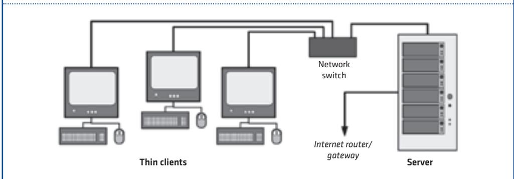
them as thin clients. Much of the expense of the upgrade is the cost of the powerful server which runs the system. Then, as the older clients fail or become unserviceable, they can be replaced with cheaper purpose-designed thin clients, further reducing the power consumption of the system.
